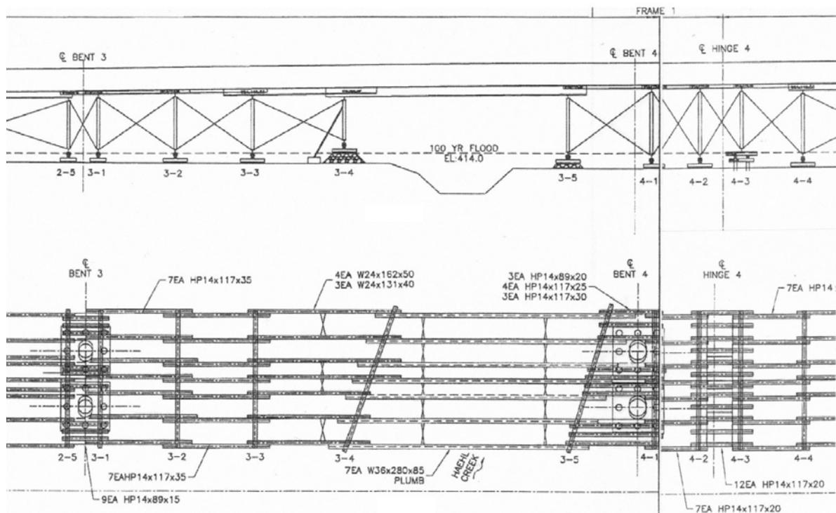
**Figure 1: Falsework Span 3 to Hinge 4**
